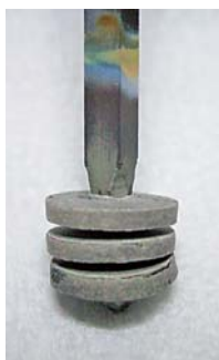
Fig. 4-3. Photographs of the SiO 2 contacting electrodes; A donut-shaped pellet made from SiO 2 powder is fixed to a polycrystalline Si rod.
